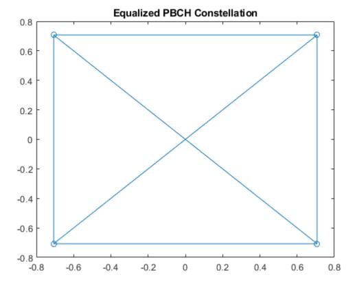
Retrieve softbits by performing PBCH decoding on the equalized symbols. pbchBits = nrPBCHDecode(pbchEqSym,ncellid,v)
