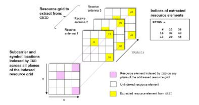
The following diagram shows the extraction process for a 4-D channel estimate grid. The number of receive antennas R = 3 and the number of antenna ports P = 2. The 4-D resource grid consists of P *M*-by-*N*-by-*R* arrays, each associated with an antenna port. Resource elements are extracted from all planes within these arrays.
