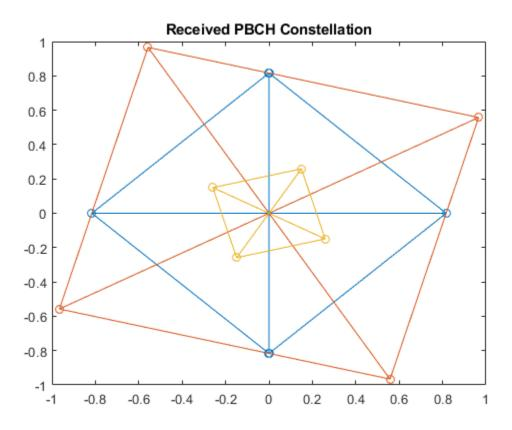
Equalize the symbols by performing MMSE equalization on the extracted resources. Plot the results.
