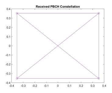
Decode the PBCH with the extracted resource elements. Plot the equalized PBCH constellation.
