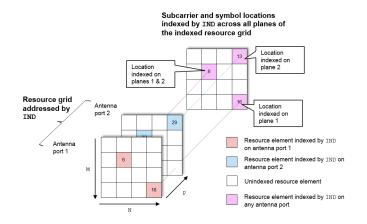
The following diagrams illustrate the resource element extraction from a 3-D received grid, where the number of receive antennas R = 3. Resource elements are extracted from the grid at the symbol and subcarrier locations.
